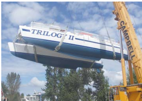
Photo above - The Trilogy was also launched by Campbell Crane, in the summer of 2010. The design uses shallow full-length keels to prevent leeway and protect the rudders. Photo right - Maui Dive Shop arranged for these two wonderful local hula dancers to perform with accompaniment at the launch ceremony, which really gave the event a Polynesian feel. Photo below - The Teralani 3 is a 65' Hughes cat based in Hawaii that is very similar to Alii Nui.
